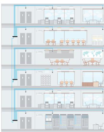
Using hybrid cabling in risers, IP and PoE for critical monitoring and security devices can be readily provided throughout a high-rise, large building, or campus of buildings.
