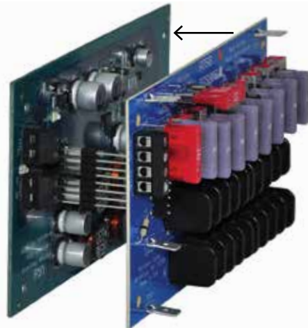
Stackable sub-assemblies save valuable enclosure space, allowing for more power distribution and access controllers.
