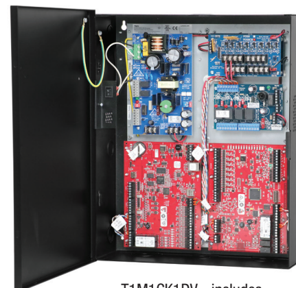
T1M1CK1DV - includes eFlow4NBV, PDS8CB, VR6, ACM4CB, wire harnesses and wire magnets
