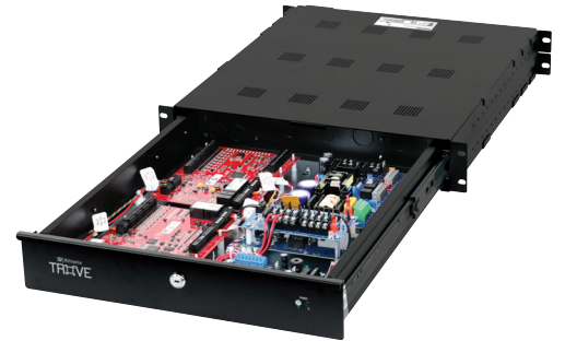
T1RM3CK1D - includes eFlow6NB, ACM4CB, VR6, PDS8CB, wire harnesses and management
