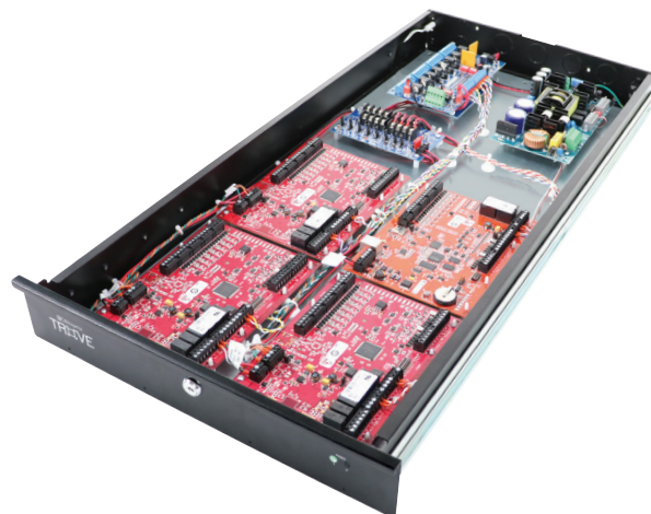
T2RM7CK1DV - includes eFlow104NBV, ACMS8CB, VR6, PDS8CB, wire harnesses and management
