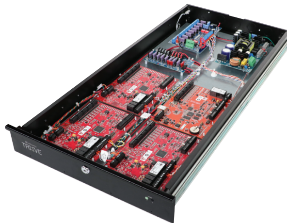
T2RM7CK1V - includes eFlow104NBV, ACMS8, VR6, PDS8, wire harnesses and management
