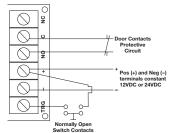
For this application Switch #1 should be in the OFF position and Switch #4 should be in the ON position.
