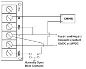
For this application Switch #1 and Switch #4 should be in the OFF position.
