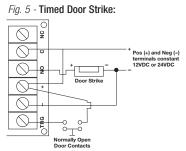
For this application Switch #1 should be in the OFF position and Switch #4 should be in the ON position.
