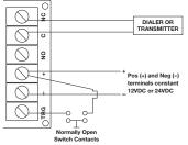
For this application Switch #1 and Switch #4 should be in the OFF position.
