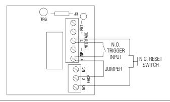
Fig. 6 Normally Closed - Non-Latching FACP trigger input:
