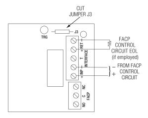
Fig. 4 Normally Open - Non-Latching FACP trigger input:
