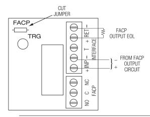
Fig. 5 Normally Open: Non-Latching FACP trigger input:
