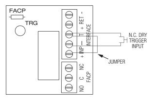
Fig. 8 Normally Closed: Latching FACP trigger input with reset (This output has not been evaluated by UL):
