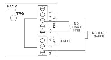
Fig. 7 Normally Closed: Non-Latching FACP trigger input:
