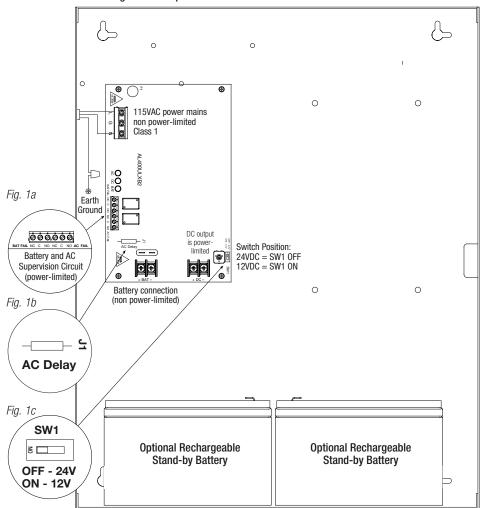
CAUTION: Optional rechargeable stand-by batteries must match the power supply output voltage setting.
