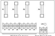
DC Output to devices 1P-4P Power Outputs, 1N-4N Common Outputs From Power Supply Board (Factory Installed)
