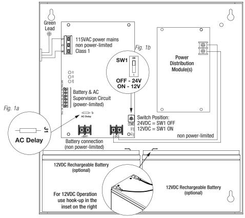
CAUTION: When power supply board is set for 12VDC use only one (1) 12VDC stand-by battery. Keep power-limited wiring separate from non power-limited. Use minimum 0.25" spacing.
