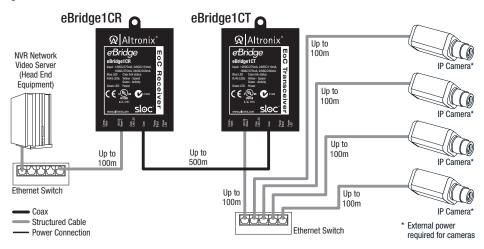
\*Note: Multiple cameras require higher bandwidth and headend equipment processing speed. It is advised to test this configuration. eBridge is rated to pass 25Mbps of data at distances up to 500m. With proper headend equipment multiple Megapixel cameras can be used.
