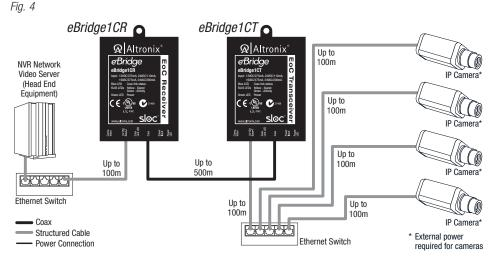
\*Note: Multiple cameras require higher bandwidth and headend equipment processing speed. It is advised to test this configuration. eBridge is rated to pass 25Mbps of data at distances up to 500m. With proper headend equipment multiple Megapixel cameras can be used.
