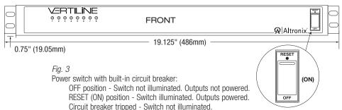
Power LEDs on faceplate are not illuminated. Outputs not powered. To reset circuit breaker set power switch to the ON (RESET) position (Fig. 3, pg. 6).
