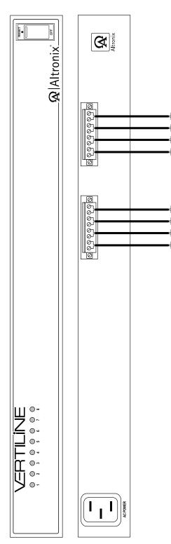
12VDC (VertiLine3D) or 24VDC (VertiLine6D) Power Outputs to Devices
