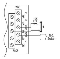
Fig. 15 - Normally Open trigger input (Non-Latching).
