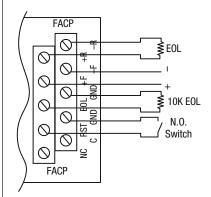
Fig. 13 - Normally Closed trigger input (Non-Latching).
