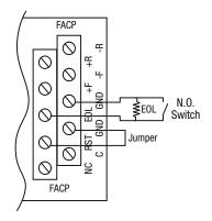
Fig. 16 - Normally Open trigger input (Latching).
