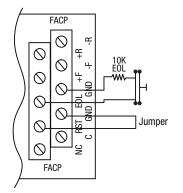
Fig. 14 - Normally Closed trigger input (Latching).
