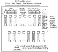
Fig. 4b - PD16WCB Power Distribution Board Power-Limited Outputs
