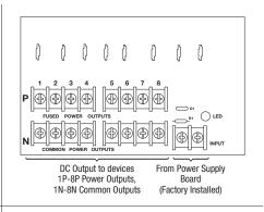
Fig. 4a - PD16W Power Distribution Board
