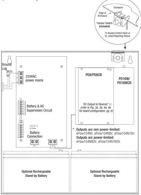
CAUTION: Power supply board is factory set for 24VDC. Use two (2) 12VDC stand-by batteries.
