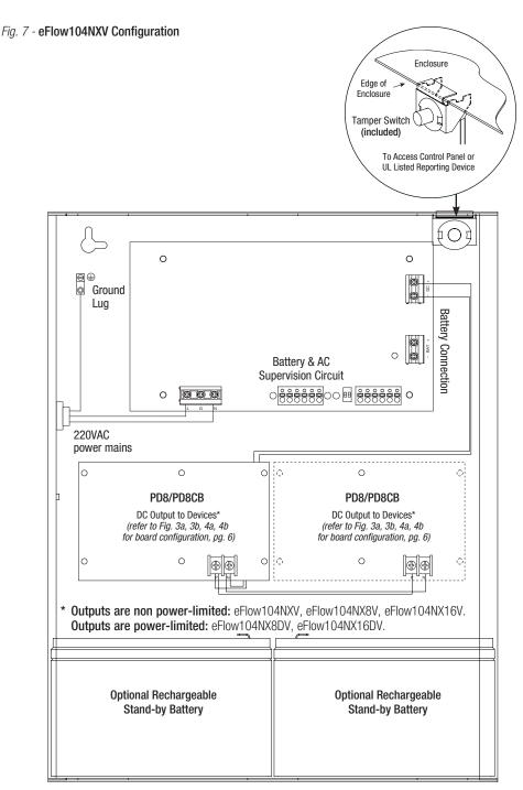
CAUTION: Power supply board is factory set for 24VDC. Use two (2) 12VDC stand-by batteries. Keep power-limited wiring separate from non power-limited. Use minimum 0.25" spacing. 12AH Rechargeable batteries are the largest batteries that can fit in this enclosure. A UL listed external battery enclosure must be used if using 40AH or 65AH batteries.
