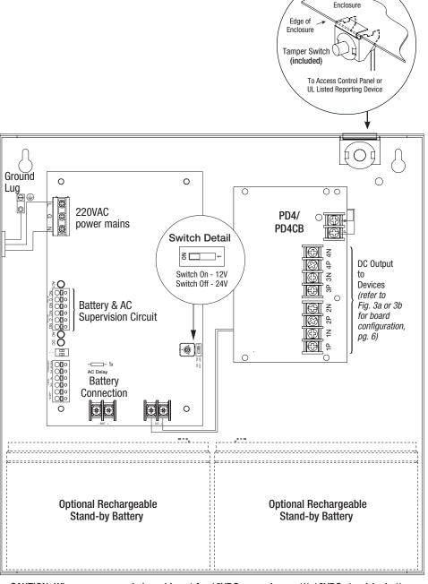
CAUTION: When power supply board is set for 12VDC use only one (1) 12VDC stand-by battery.
