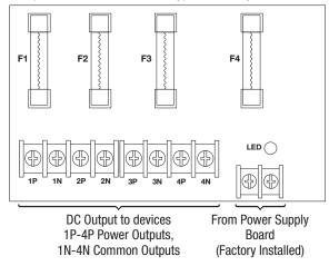
Fig. 3b - PD4CB Power Distribution Board
