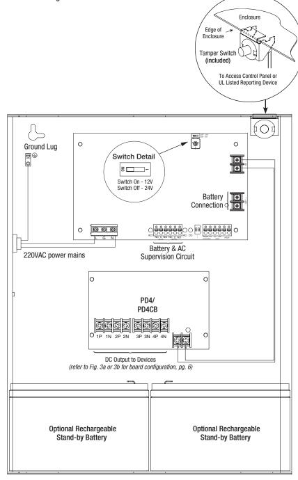
CAUTION: When power supply board is set for 12VDC use only one (1) 12VDC stand-by battery. Keep power-limited wiring separate from non power-limited. Use minimum 0.25" spacing. 12AH Rechargeable batteries are the largest batteries that can fit in this enclosure. A UL listed external battery enclosure must be used if using 40AH or 65AH batteries.
