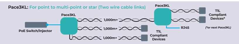
The above scheme shows the first Pace3KL in a typical star configuration, while the second Pace3KL shows how to configure for a continued multi-point drop-off using additional TIL switch to connect TIL compliant devices in multiple locations.
