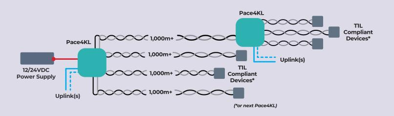
The Pace4KL T1L adaptor/switch can connect directly to up to four 3cg, T1L devices and feature dual network uplink ports. An additional Pace4KL can be added to the remote end to connect more compliant devices. Network managed versions allow for control, monitoring, and reporting of power diagnostics and feature a single network uplink port.
