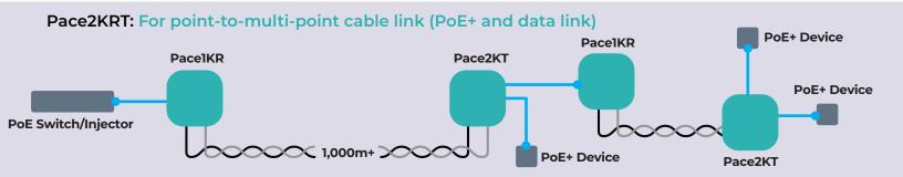
In the above setups the remote end device/s can operate with POE enabled or not. If enabled, remote power supply is not required. POE can also deliver power more efficiently than SPoE Classes 10-12.
